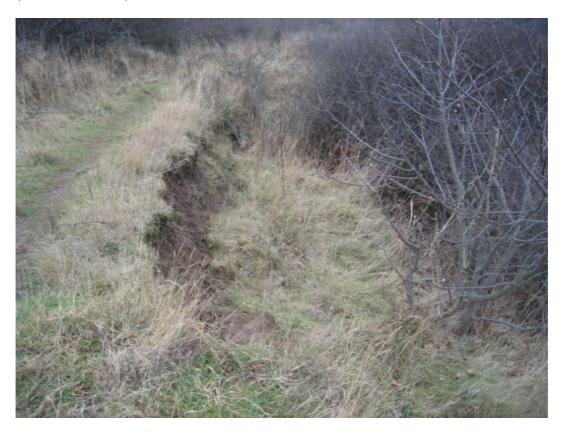
Plate 10 Site view of mid-slope back rotated block and surface tension crack development (January 2010).
